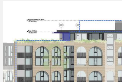
Encroaching eaves to the east
